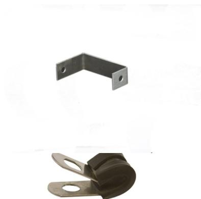
It is recommended that fixings should be placed at intervals of no more than 1.2m apart. Where cable ties are used they should be used in conjunction with a neoprene sleeve and not over tightened to prevent damage to the outer sleeve of the LHD. Minimum bend radius of digital LHD is 50mm (100mm in cold store environments). Local regulations should always be adhered to.
